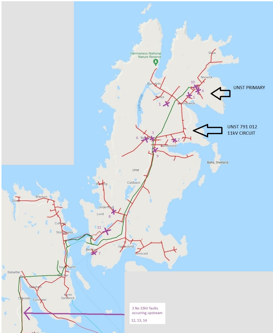
Figure 2: Location of faults affecting Unst customers
