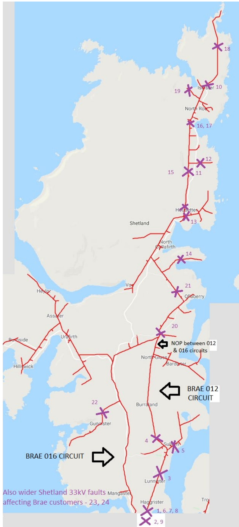
Figure 2: Location of faults affecting Brae 012 & 016 customers
