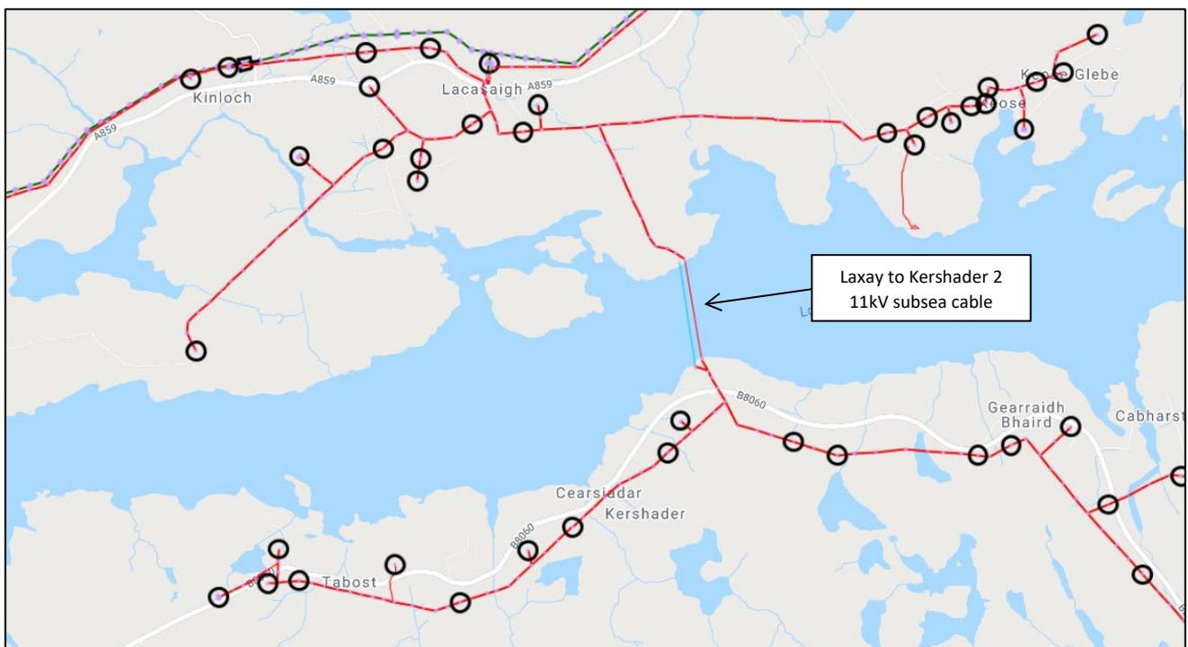
Previously, a second subsea cable was in operation adjacent to the existing cable. That cable has been decommissioned following an electrical fault from abrasive wear, however the 11kV onshore switching assets remain in place.
