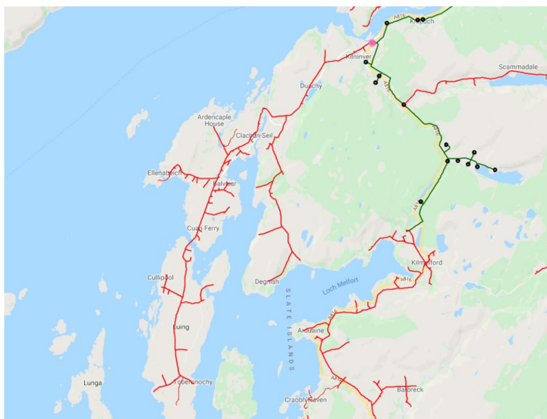
Figure 4: The 11kV Network Fed from Kilniver.
